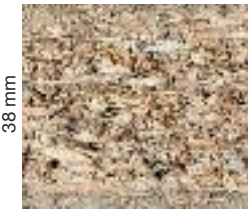
Truciolare: spessore 38 mm Chipboard panel: panel thickness 38 mm
